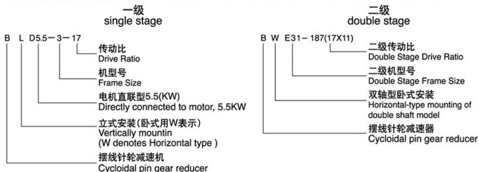
B系列(等同机械部标准) B series (equivalent to Standard of Ministry of Machine-Building Industry)
